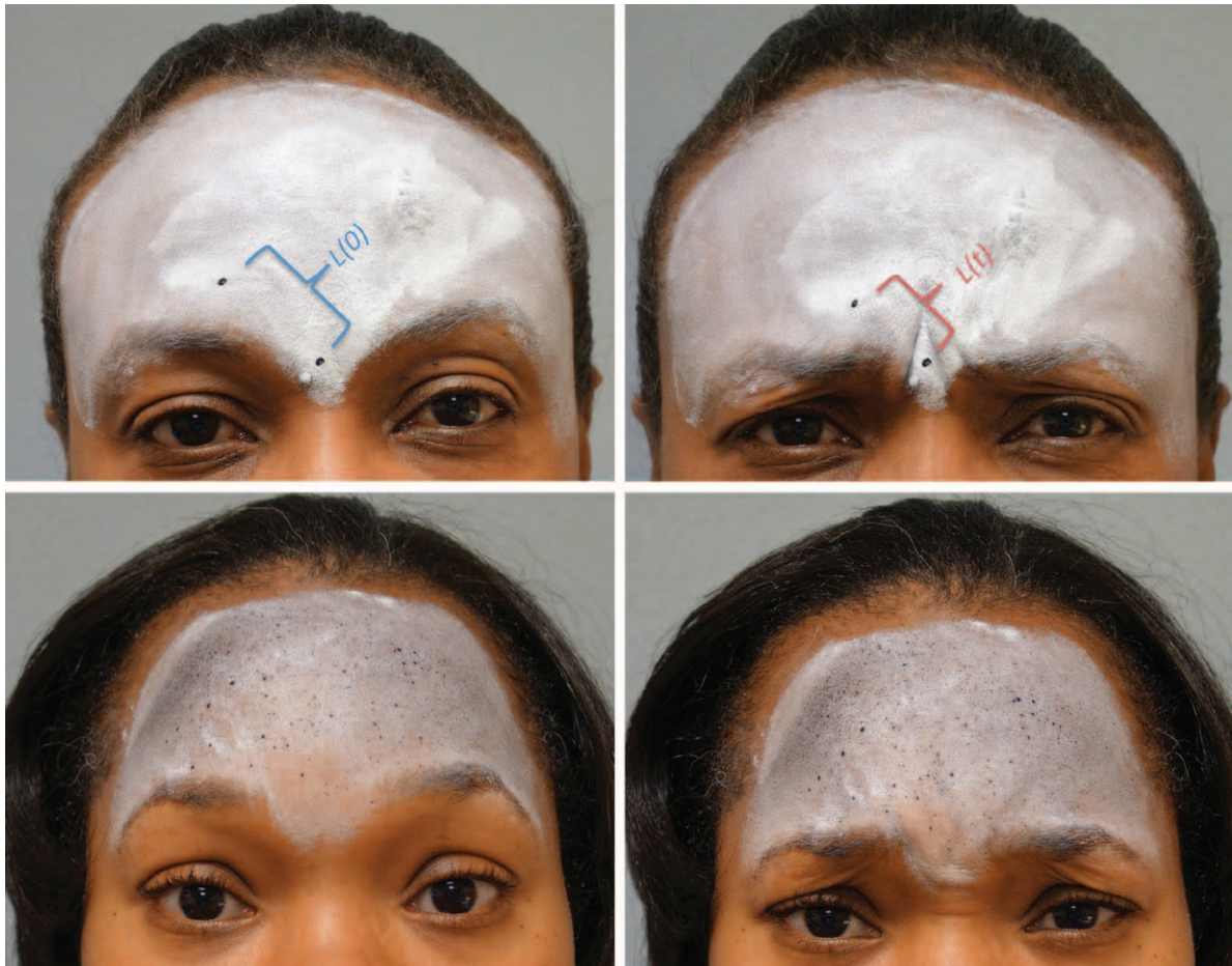
Fig. 1. The concept of speckle tracking with digital image correlation is illustrated here. Digital image correlation precisely captures the change in dynamic tissue strain through speckle displacement. (Above, left) A patient is illustrated with the white foundation makeup and two speckles. At rest, there is a set length between the two speckles, L(0) . (Above, right) Following corrugator activation, the distance between the two speckles changes with a new length, L(t) . The strain of this tissue is the percentage change between L(0) and L(t) . (Below, left) This patient, following application of the white foundation and black speckle makeup, has the complete complement of potential data points. (Below, right) Now, with corrugator activation, strain between all the speckles relative to each other is determined over all 35 frames. These data are uploaded into ARAMIS software, where average strain is calculated.
